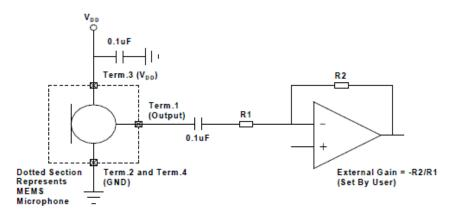
**Test Setup Drawing**
