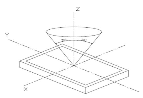
Inspection should be performed within angle  $\Phi$  ( $\Phi$  is usually 30°) from Z axis to each X and Y.
