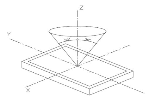
Inspection should be performed within angle  $\Phi$  ( $\Phi$  is usually 30°) from Z axis to each X and Y.
