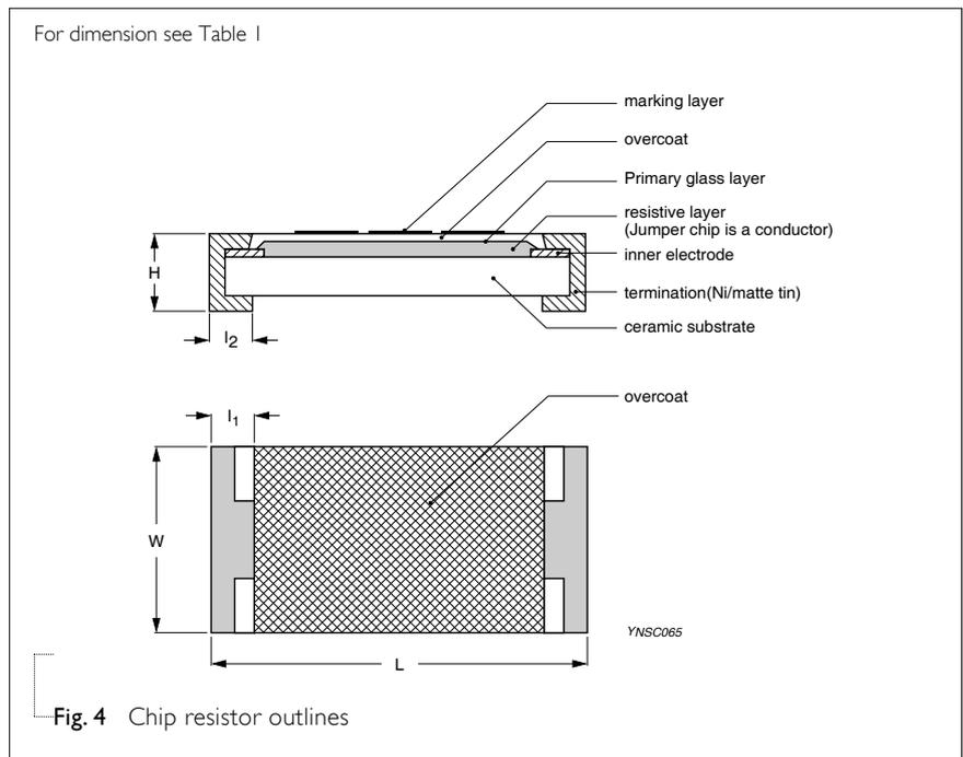
Fig. 4 Chip resistor outlines
