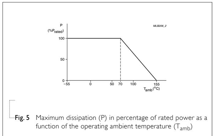
Fig. 5 Maximum dissipation (P) in percentage of rated power as a function of the operating ambient temperature (T<sub>amb</sub>)
